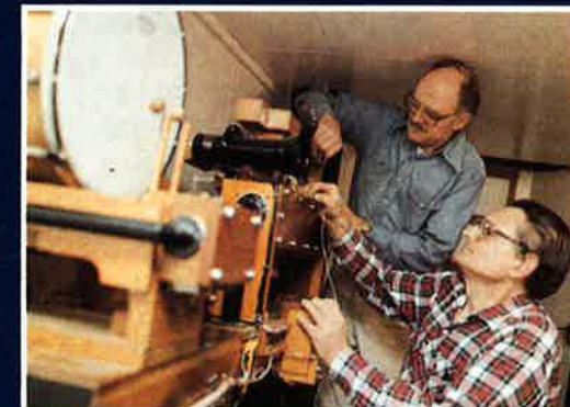
Lance Johnson and Craven Nichols wire in traps in new organ percussion chamber.
